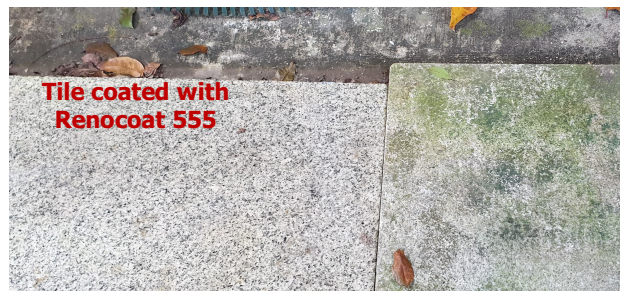
Tiles placed outdoor subject to rain & shine for 16 weeks.
